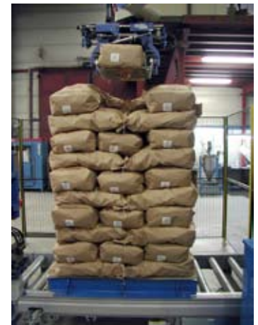
Robot palletizing of sacks, cardboard –or plastic boxes etc.
